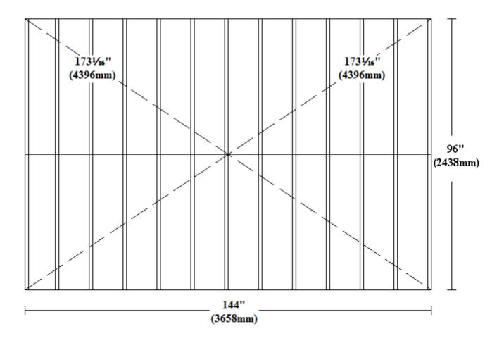
NB:- Floor joists run from gable to gable.
